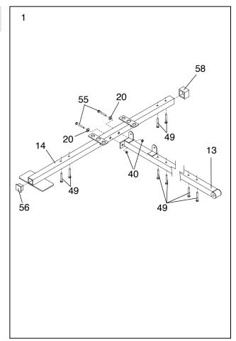
Slide the Lat Upright (1) onto the indicated 5/16" x 2 1/2" Carriage Bolts (49) in the Weight Base (14). Hand tighten two 5/16" Nylon Locknuts (40) onto the Carriage Bolts. Do not tighten the Nylon Locknuts yet.
